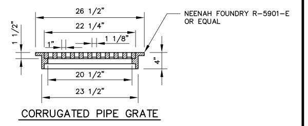
CORRUGATED PERFORATED PIPE DRYWELL WITH GRATE
