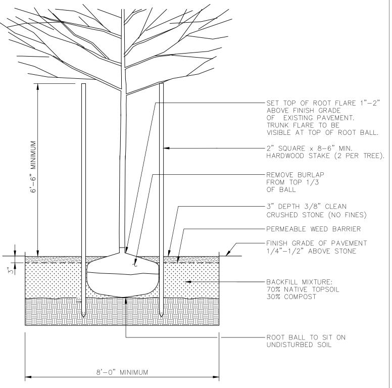
TREE PIT WITH CRUSHED STONE SURFACE
