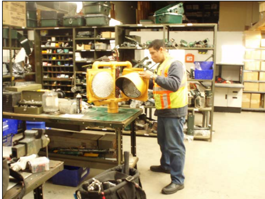
Fabrication of new traffic calming flashers.
