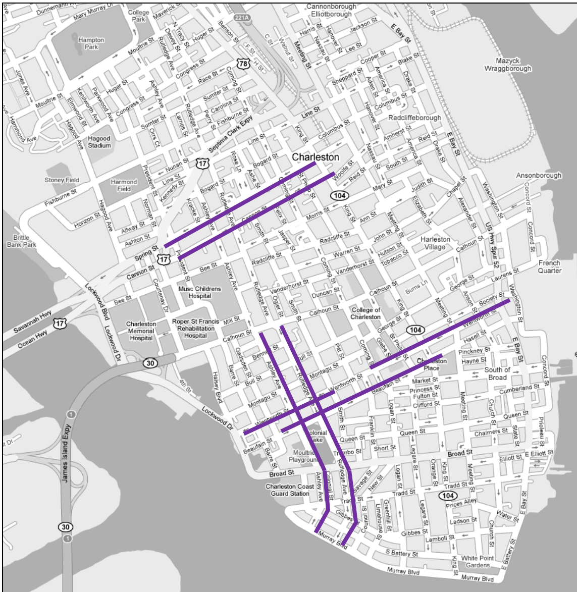
Figure 3.4 Map of Charleston, South Carolina, showing recent one-way to two-way conversions, including the couplet of Beaufain Street and Wentworth Street, Ashley Avenue and Rutledge Avenue, and Spring Street and Cannon Street.
